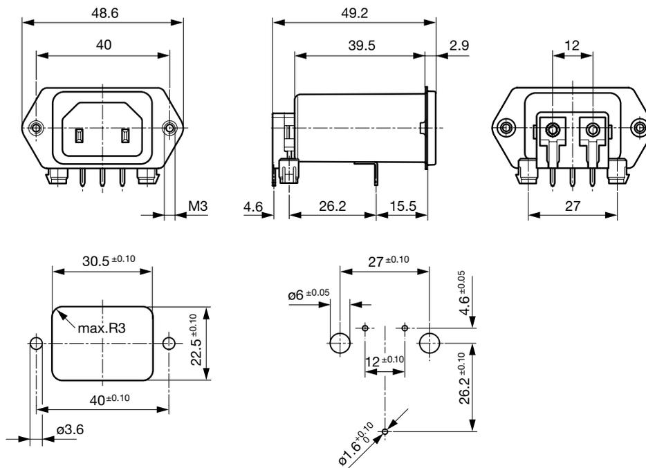
PCB rear side mounting, protection class I
