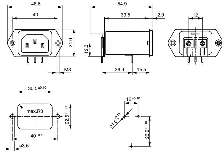
Screw and snap-in mounting with flexible wire
